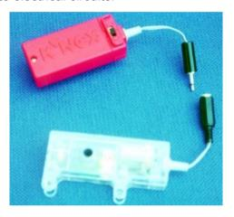
The switch built into the battery pack can be used to turn the power on and off, and to reverse the polarity of the wires.
