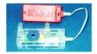
Connecting a battery motor to your model can be achieved by putting rods through the four holes at the edge of the case (see picture opposite for one way to do it). The battery pack may also be attached in a similar way. It may take a bit of practice before you become proficient at this.
