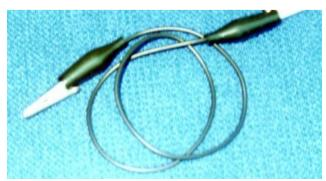
The crocodile clips have plastic sleeves over them, so as to prevent accidental short circuits. We find it best to slide the plastic sleeves off for
